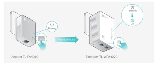
Pair Adapter and Extender B by referring to step 3. Extender B will automatically sync Wi-Fi settings from Extender A.
